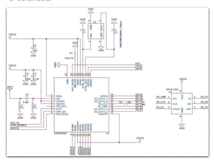
Figure 4 Schematics of Esp-12E WiFi Module
