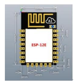
Figure 4 Top View of ESP-12E WiFi Module
