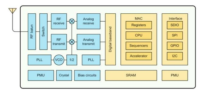
Figure 1 ESP8266EX Block Diagram
