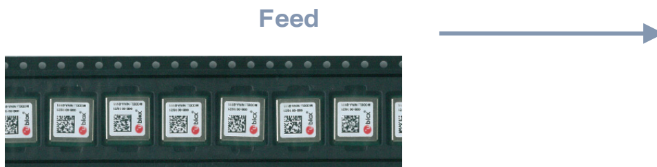
Figure 7: Orientation of NINA-W101 module on tape
