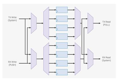
Another example is a UART: because the TX/CTS and RX/RTS parts a of a UART are asynchronous, they are
