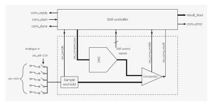
The ADC requires a 48MHz clock (clk\_adc), which could come from the USB PLL. Capturing a sample takes 96 clock cycles (96 x 1 / 48MHz) = 2 µs per sample (500kS/s). The clock must be set up correctly before enabling the ADC.
