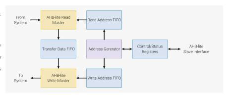
The DMA can perform one read access and one write access, up to 32 bits in size, every clock cycle. There are 12 independent channels, each which supervise a sequence of bus transfers, usually in one of the following scenarios:
