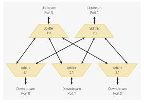
The crossbar is built from two components:
