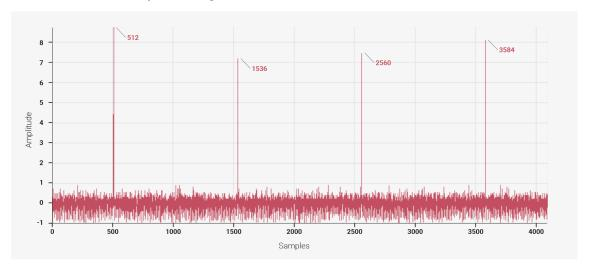
The INL and DNL errors come from an error in the scaling of some internal capacitors of the ADC. These capacitors are small in value (only tens of femto Farads) and at these very small values, chip simulation of these capacitors can deviate slightly from reality. If these capacitors had matched correctly, the ADCs performance could have been better.
