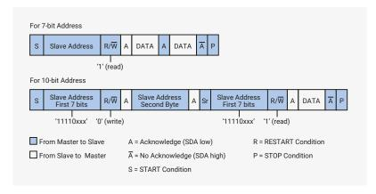
When a master does not want to relinquish the bus with a STOP condition, the master can issue a RESTART condition. This is identical to a START condition except it occurs after the ACK pulse. Operating in master mode, the DW\_apb\_i2c can then communicate with the same slave using a transfer of a different direction. For a description of the combined format transactions that the DW\_apb\_i2c supports, refer to Section 4.3.5.2.
