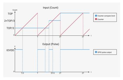
The behaviour becomes even more perplexing if the TOP register is also modified. It would be difficult for software to write to CC or TOP with the correct timing. To solve this, each slice has two copies of the CC and TOP registers: one copy which software can modify, and another, internal copy which is updated from the first register at the instant the counter wraps. Software can modify its copy of the register at will, but the changes are not captured by the PWM output until the next wrap.
