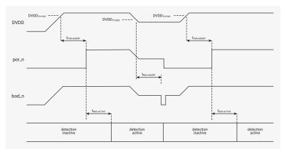
Once the chip is out of reset, detection can be disabled under software control. This also saves a small amount of power. If detection is subsequently re-enabled, there will be another short delay, the *brown-out detection enable delay* ( $t_{\text{BOD.ENABLE}}$ ), before it becomes active again. This is shown in Figure 25.
