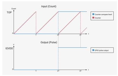
A CC value of 0 will produce a 0% output, i.e. the output signal is always low. A CC value of TOP + 1 (i.e. equal to the period, in non-phase-correct mode) will produce a 100% output. For example, if TOP is programmed to 254, the counter will have a period of 255 cycles, and CC values in the range of 0 to 255 inclusive will produce duty cycles in the range 0% to 100% inclusive.
