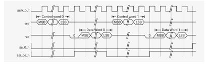
The only modification needed to perform a continuous nonsequential transfer is to write more control words into the transmit FIFO buffer; this is illustrated in Figure 137. In this example, two data words are read from the external serial-slave device.
