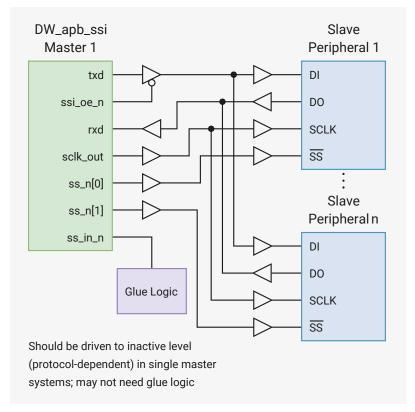
The serial bit-rate clock, generated and controlled by the DW\_apb\_ssi, is driven out on the sclk\_out line. When the DW\_apb\_ssi is disabled (SSI\_EN = 0), no serial transfers can occur and sclk\_out is held in "inactive" state, as defined by the serial protocol under which it operates.
