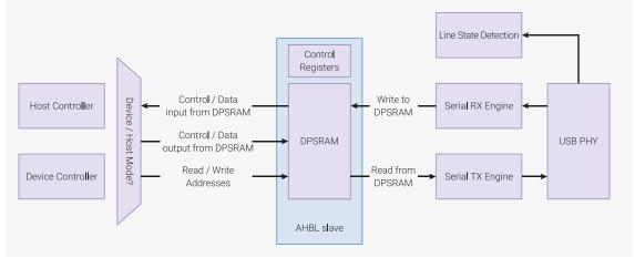
The USB controller is an area efficient design that muxes a device controller or host controller onto a common set of components. Each component is detailed below.
