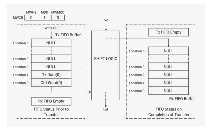
Continuous transfers occur as shown in Figure 142, with the control word for the next transfer following immediately after the LSB of the current data word.
