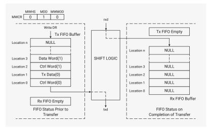
The Microwire handshaking interface can also be enabled for DW\_apb\_ssi master write operations to external serial-slave devices. To enable the handshaking interface, you must write 1 into the MHS bit field (bit 2) on the MWCR register. When MHS is set to 1, the DW\_apb\_ssi serial master checks for a ready status from the slave device before completing the transfer, or transmitting the next control word for continuous transfers.
