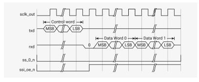
Figure 139. FIFO Status for Sequential Microwire Transfer (receiving data frame)
