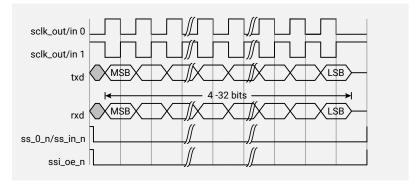
Continuous data frames are transferred in the same way as single frames, with the MSB of the next frame following directly after the LSB of the current frame. The slave select signal is held active for the duration of the transfer.
