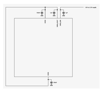
The regulator must have 1µF capacitors placed close to its input (VREG\_VIN) and output (VREG\_VOUT) pins.
