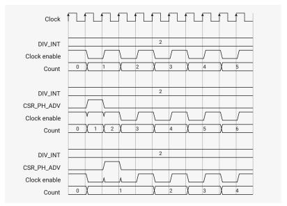
The counter can not count faster than once per cycle, so PH\_ADV requires DIV\_INT > 1 or DIV\_FRAC > 0. Likewise, the counter will not start to count backward if PH\_RET is asserted when the clock enable is permanently low.
