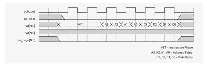
Figure 159 describes a DDR write transfer where instruction, address and data all are transferred in DDR format.
