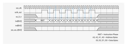
Figure 162. Transmit Data With DDR\_DRIVE\_EDGE = 2
