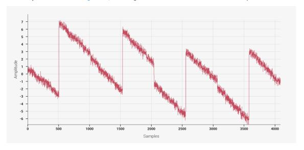
Nominally an ADC moves from one digital value to the next digital value, colloquially expressed as "no missing codes". However, if the ADC skips a value bin this would cause a spike in the Differential Non-Linearity (DNL) error. These types of error often only occur at specific codes due to the design of the ADC.
