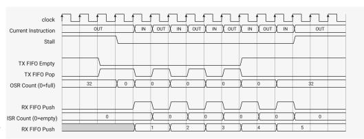
To trigger automatic push or pull at the correct time, the state machine tracks the total shift count of the ISR and OSR, using a pair of saturating 6-bit counters.
