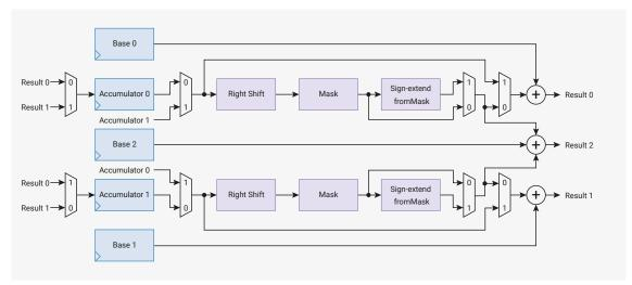
The processor can write or read any interpolator register in one cycle, and the results are ready on the next cycle. The processor can also perform an addition on one of the two accumulators ACCUM0 or ACCUM1 by writing to the corresponding ACCUMx\_ADD register.
