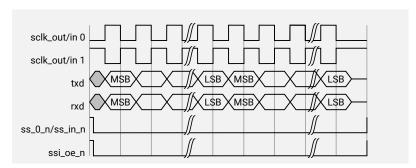
There are four possible transfer modes on the DW\_apb\_ssi for performing SPI serial transactions. For transmit and receive transfers (transfer mode field (9:8) of the Control Register 0 = 00b), data transmitted from the DW\_apb\_ssi to the external serial device is written into the transmit FIFO. Data received from the external serial device into the DW\_apb\_ssi is pushed into the receive FIFO.
