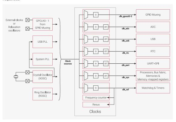
For very low cost or low power applications where precise timing is not required, the chip can be run from the internal Ring Oscillator (ROSC). Alternatively the user can provide external clocks or construct simple relaxation oscillators using the GPIOs and appropriate external passive components. Where timing is more critical, the Crystal Oscillator (XOSC) can provide an accurate reference to the 2 on-chip PLLs to provide fast clocking at precise frequencies.
