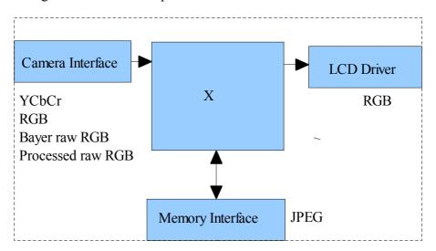
The data format at LCD driver are always RGB. For example, RGB444, RGB565, RGB555, RGB888 etc. The data format and memory interface are always Compressed. The Compression data is compressed from YCbCr data. So Both RGB and YCbCr data are needed inside the backend chip. The "X" block is different for different backend chips.
