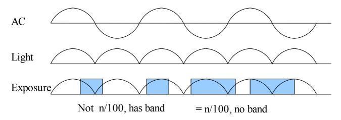
The strength of office light is not even. It changes with AC frequency. For example, if the AC frequency is 50Hz, the light changes strength at 100hz.
