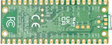
Raspberry Pi Pico W has been designed to be a low cost yet flexible development platform for RP2040, with the addition of a 2.4GHz wireless interface and the following key features:
