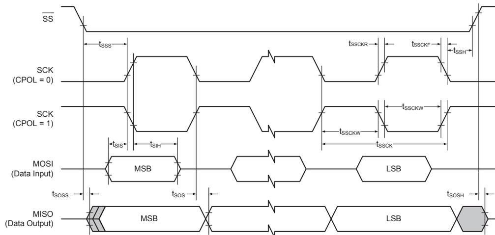
Table 34-19. USART in SPI Mode - Timing Characteristics
