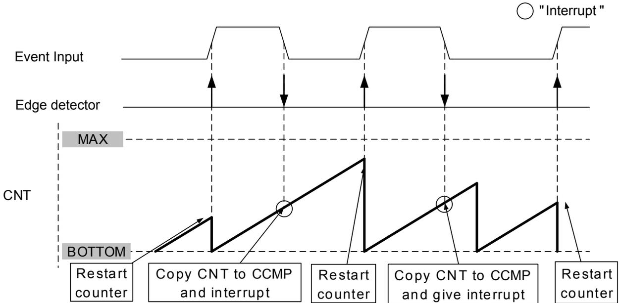
**Input Capture Frequency and Pulse Width Measurement Mode**
