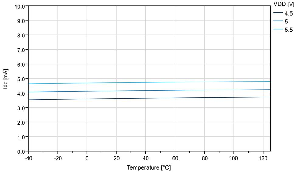
**Figure 35-24. ATtiny814: Idle Supply Current vs. V<sub>DD</sub> (f=32KHz OSCULP32K)**
