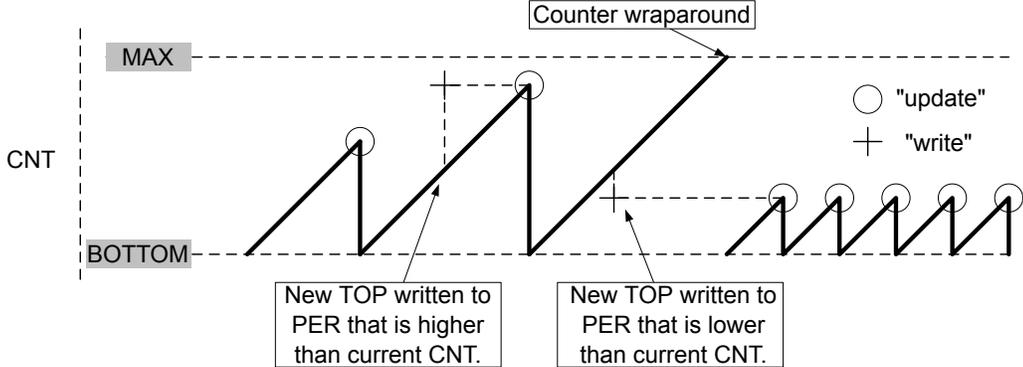
A counter wraparound can occur in any mode of operation when up-counting without buffering. This is due to the fact that the registers TCA.CNT and TCA.PER are continuously compared: if a new TOP value is written to TCA.PER that is lower than current TCA.CNT, the counter will wrap first before a compare match happened.
