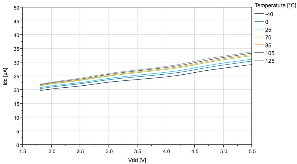
**Figure 35-51. BOD Current vs.  $V_{DD}$  (Sampled BOD at 125Hz)**
