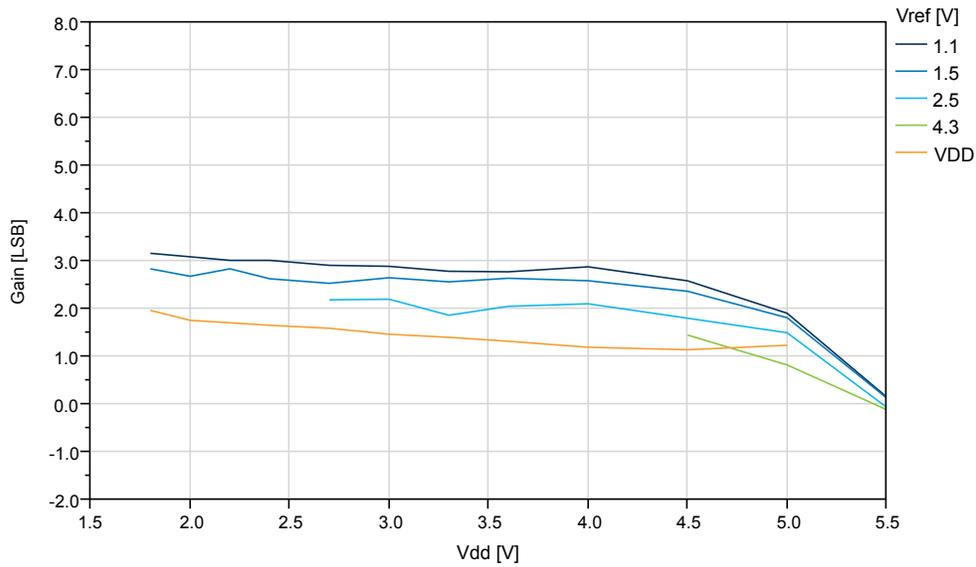
**Figure 35-61. Gain Error vs.  $V_{ref}$  ( $V_{DD}=5.0V$ , 115kps)**
