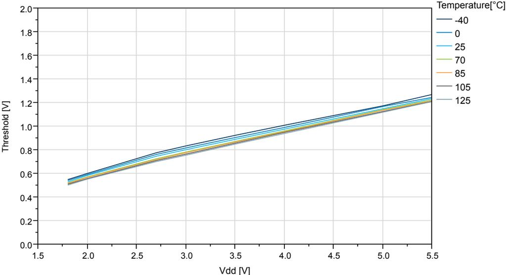
Figure 35-32. IO Pin Input Threshold Voltage vs. V<sub>DD</sub> (T=25°C)
