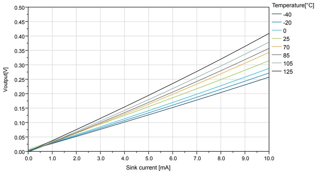
**Figure 35-37. IO Pin Output Voltage vs. Sink Current ( $V_{DD}=5.0V$ )**
