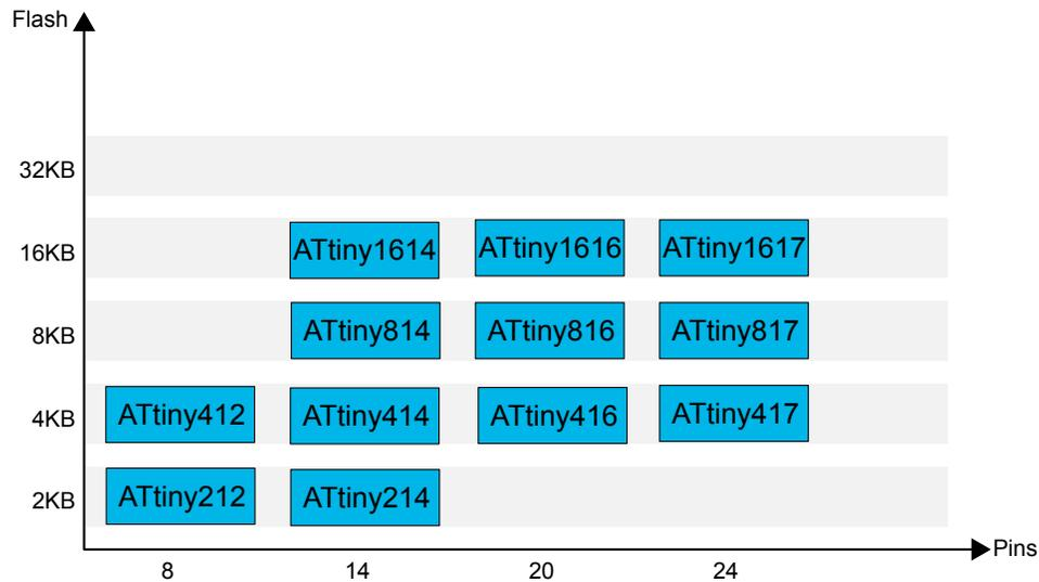
Devices with different Flash memory size typically also have different SRAM and EEPROM.
