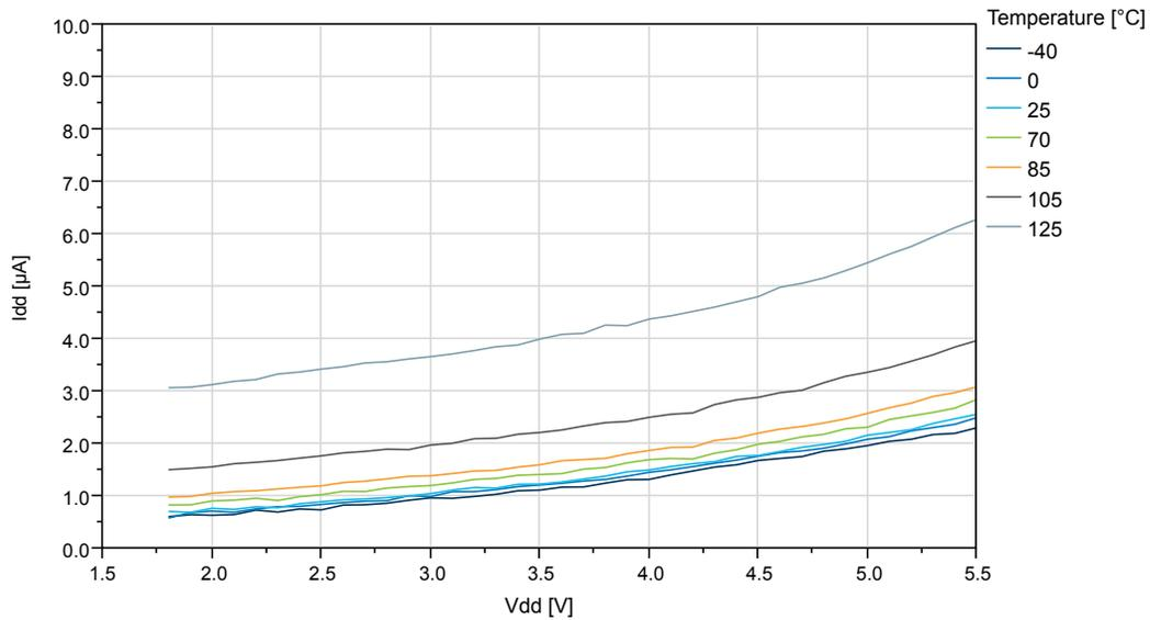
**Figure 35-29. ATtiny814: Standby Mode Supply Current vs.  $V_{DD}$  (Sampled BOD running at 125Hz)**
