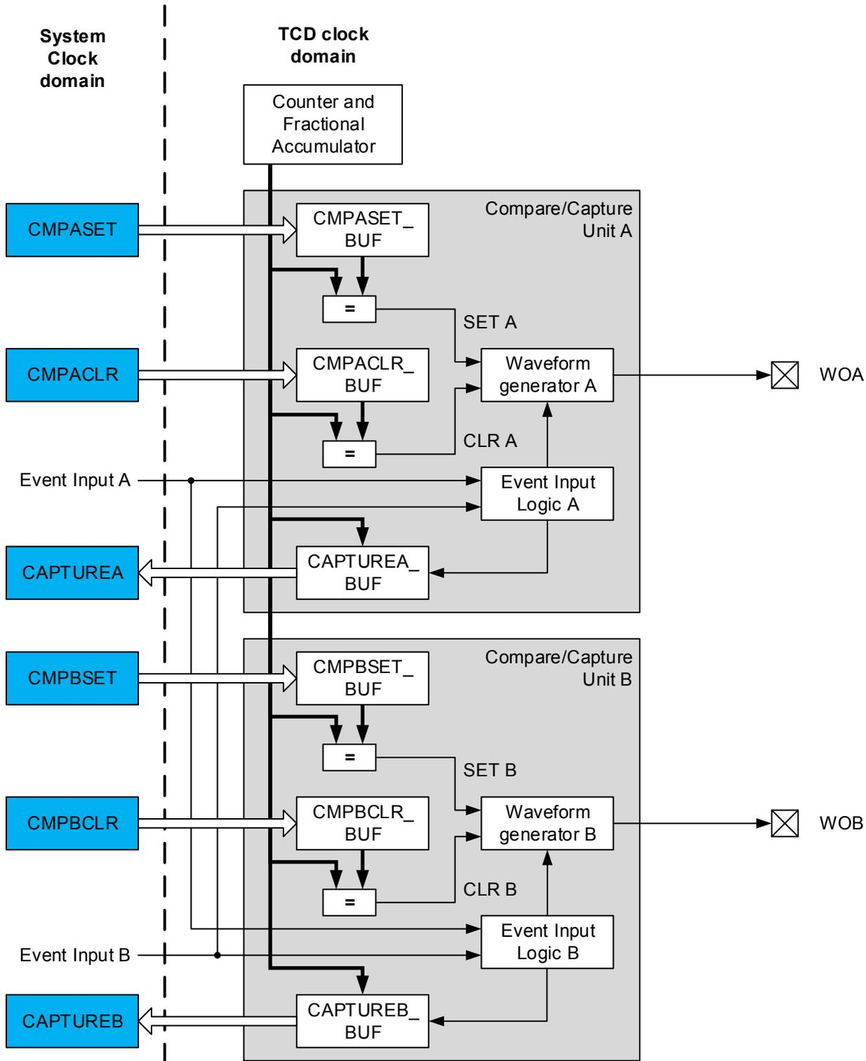
The TCD core is asynchronous to the system clock. The timer/counter consist of two compare/capture units, each with a separate waveform output. In addition there are two extra waveform outputs which can be equal to the output from one of the units. The compare registers CMPxSET, CMPxCLR are stored in
