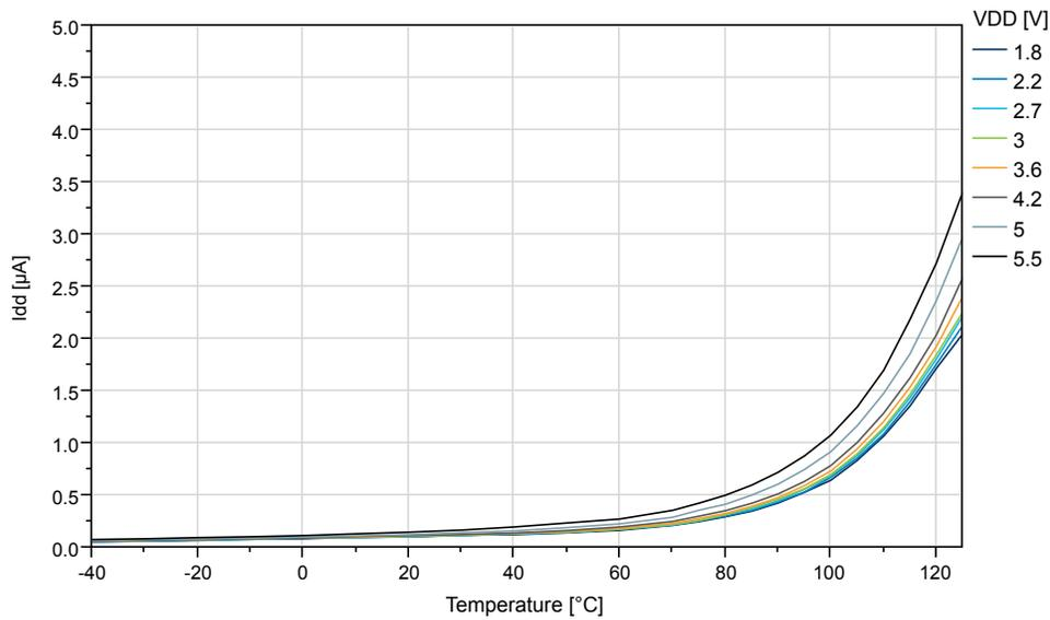
**Figure 35-11. ATtiny214/ATtiny414: Power Down Mode Supply Current vs.  $V_{DD}$  (all functions disabled)**
