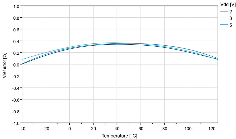
**Figure 35-47. Internal 1.1V Reference vs. Temperature**
