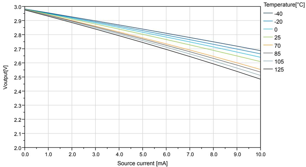
**Figure 35-41. IO Pin Output Voltage vs. Source Current ( $V_{DD}=5.0V$ )**
