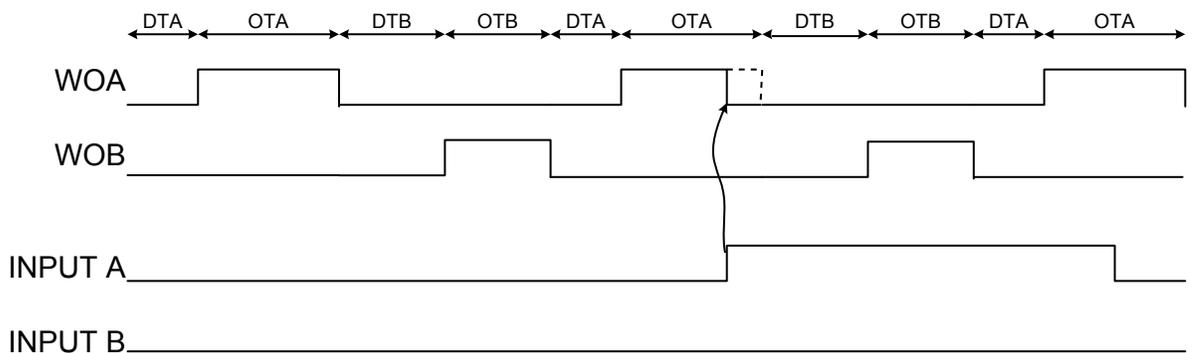
If Input mode 9 is used on input B and an positive input event occurs while in On time B, the output will be off for the rest of the on-time.
