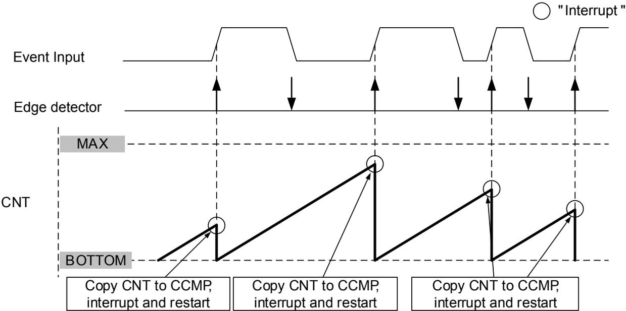
**Input Capture Pulse Width Measurement Mode**
