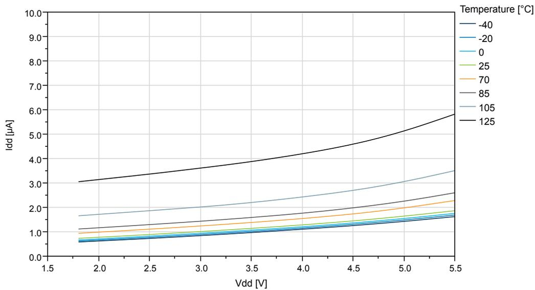
**Figure 35-13. ATtiny214/ATtiny414: Standby Mode Supply Current vs.  $V_{DD}$  (RTC running with internal OSCULP32K)**
