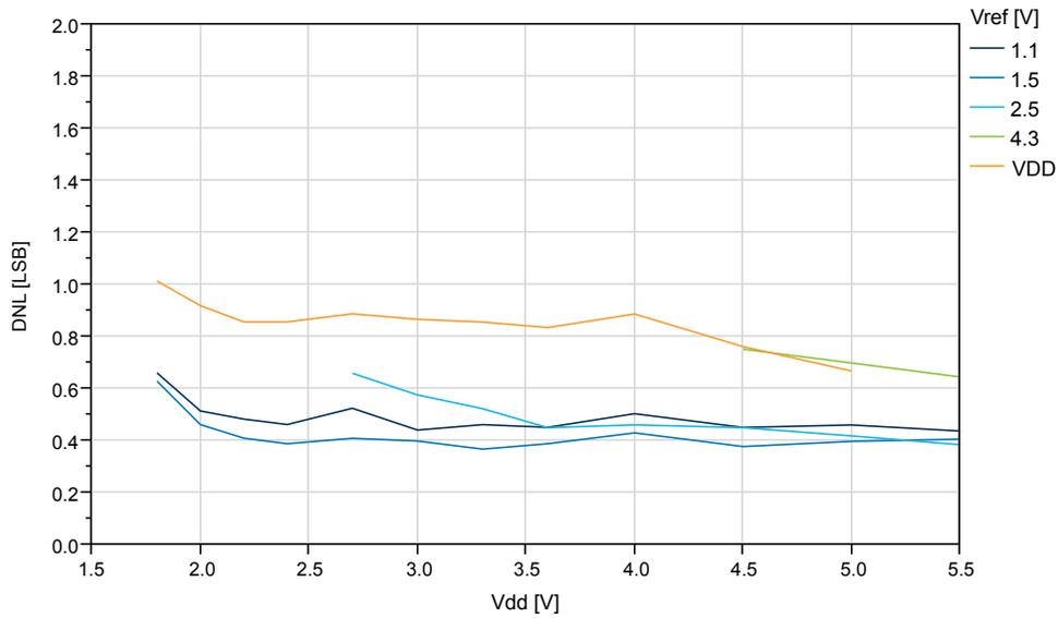
Figure 35-59. DNL vs.  $V_{ref}$  ( $V_{DD}=5.0V$ , 115ksps)
