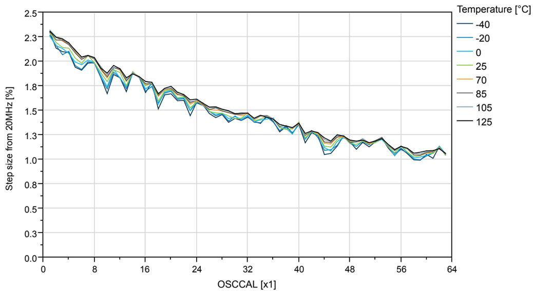
Figure 35-71. OSC20M internal Oscillator: Frequency vs. Calibration Value ( $V_{DD}=3V$ )
