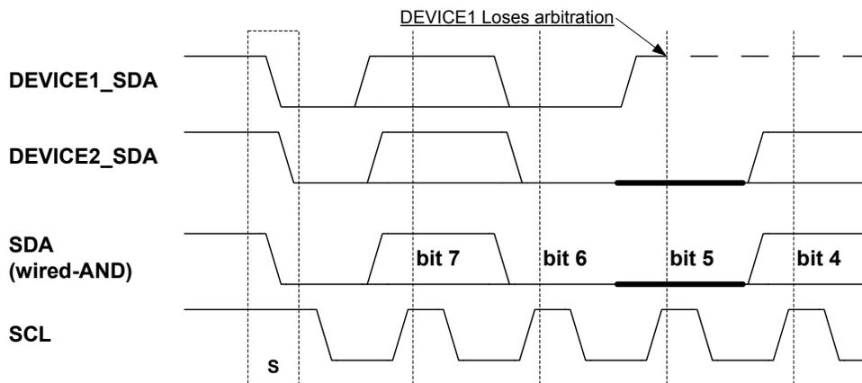
Figure 26-10 shows an example where two TWI masters are contending for bus ownership. Both devices are able to issue a START condition, but DEVICE1 loses arbitration when attempting to transmit a high level (bit 5) while DEVICE2 is transmitting a low level.
