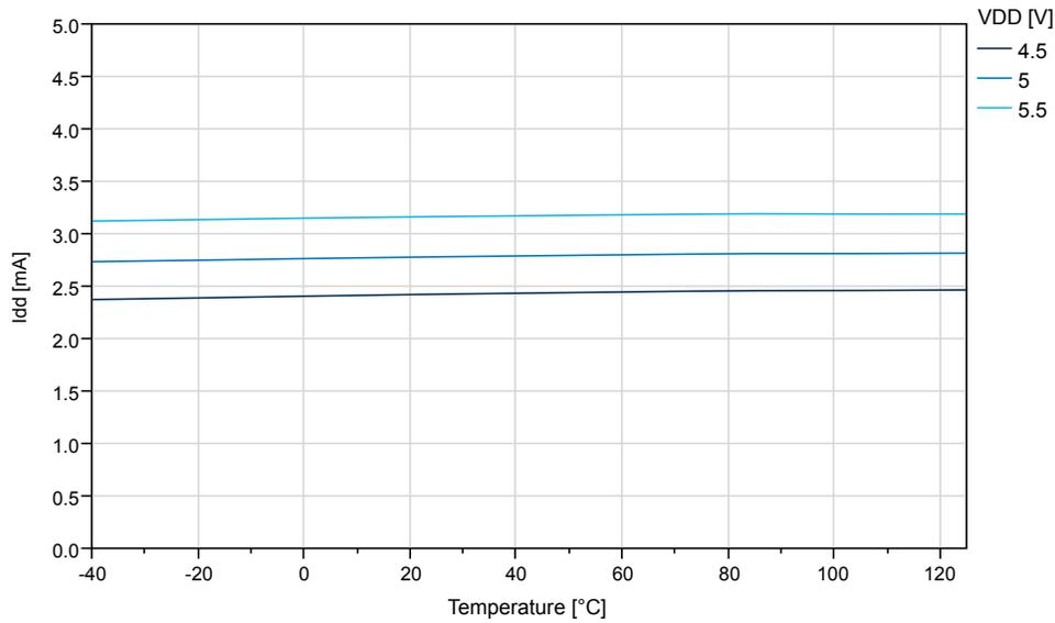
**Figure 35-9. ATtiny214/ATtiny414: Idle Supply Current vs.  $V_{DD}$  (f=32KHz OSCULP32K)**
