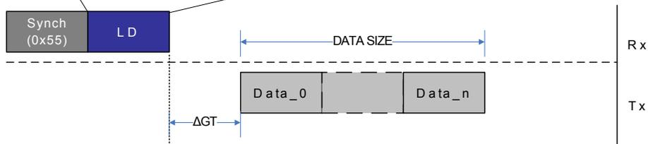
The Figure above shows an example of a typical LD sequence, where data is received after the Guard Time period. Loading data from the UPDI pointer register follows the same transmission protocol.
