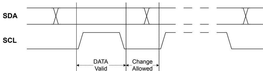
Combining bit transfers results in the formation of address and data packets. These packets consist of eight data bits (one byte) with the most-significant bit transferred first, plus a single-bit not-acknowledge (NACK) or acknowledge (ACK) response. The addressed device signals ACK by pulling the SCL line low during the ninth clock cycle, and signals NACK by leaving the line SCL high.
