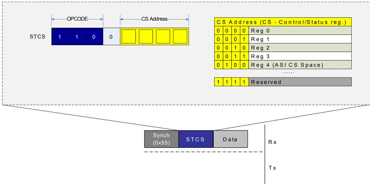
Figure 33-14 shows the data frame transmitted after the SYNCH and instruction frames. There is no response generated from the STCS instruction, as is the case for ST and STS.
