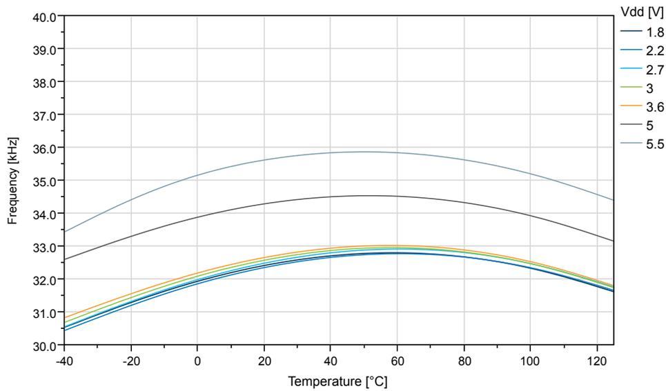
Figure 35-75. OSCULP32K Internal Oscillator Frequency vs. V<sub>DD</sub>
