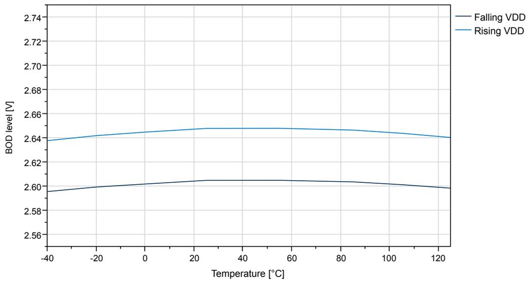
Figure 35-55. BOD Threshold vs. Temperature (Level 4.3V)
