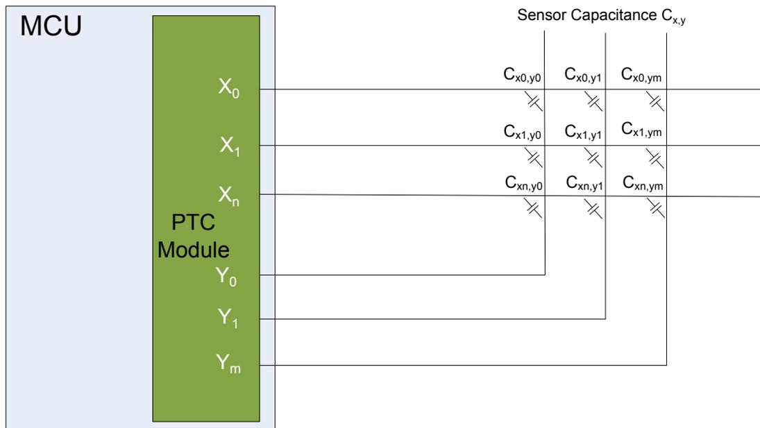
**32.5.1.2 Self-Capacitance Sensor Arrangement**
