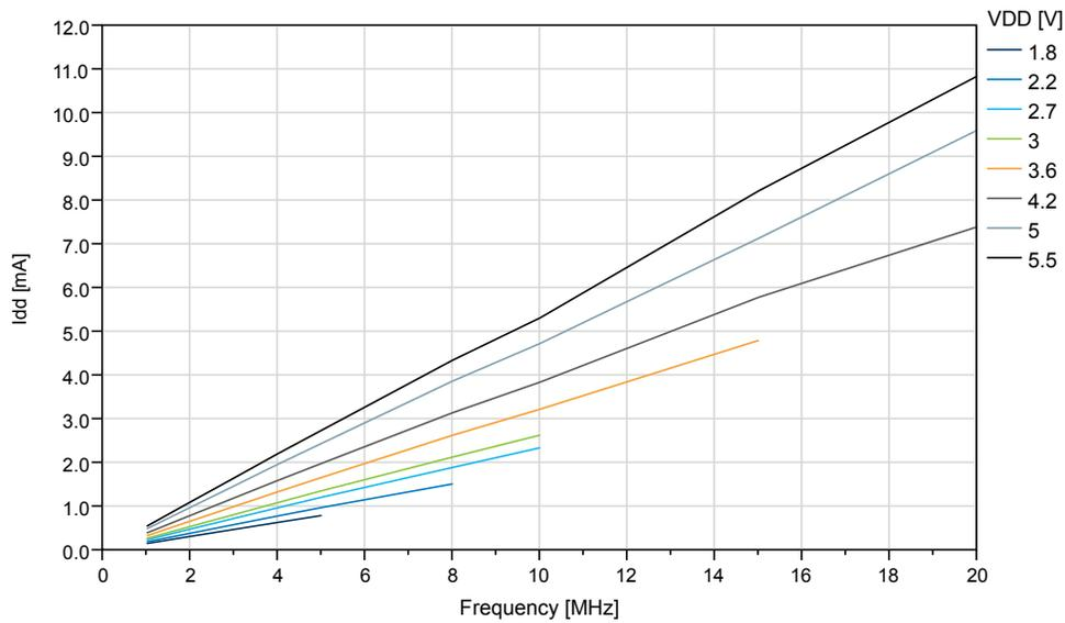
**Figure 35-17. ATtiny814: Active Supply Current vs. Frequency [0.1, 1.0]MHz at T=25°C**
