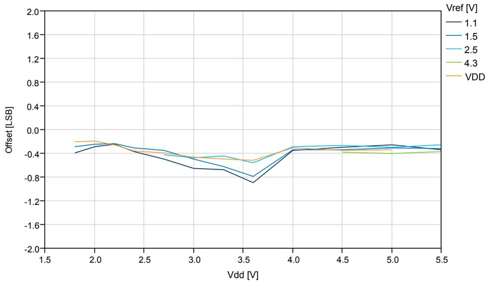
Figure 35-65. Offset Error vs.  $V_{ref}$  ( $V_{DD}=5.0V$ , 115ksps)
