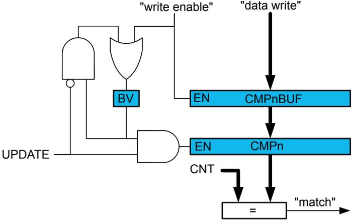
Both the TCA.CMPn and TCA.CMPnBUF registers are available as I/O registers. This allows initialization and bypassing of the buffer register and the double buffering function.
