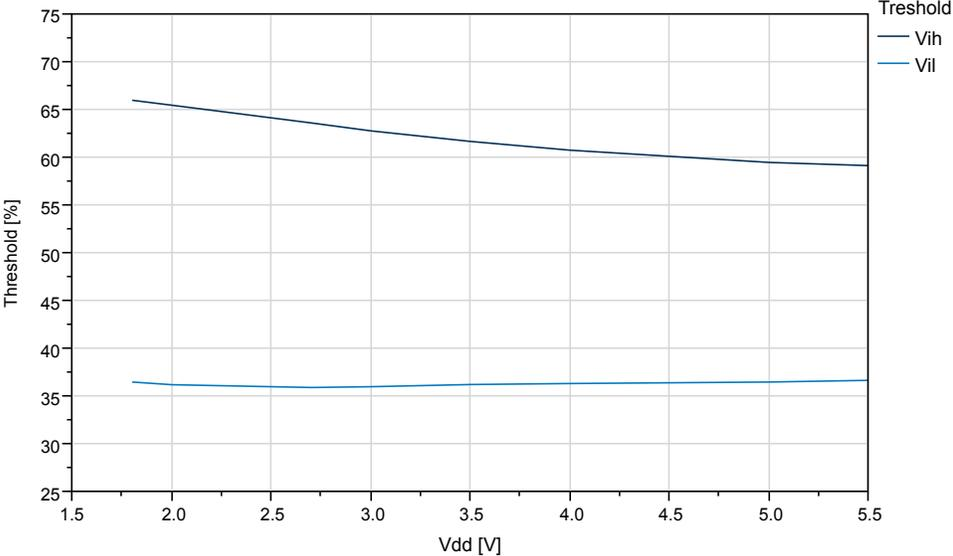
Figure 35-33. IO Pin Input Threshold Voltage vs.  $V_{DD}$  ( $V_{IH}$ )
