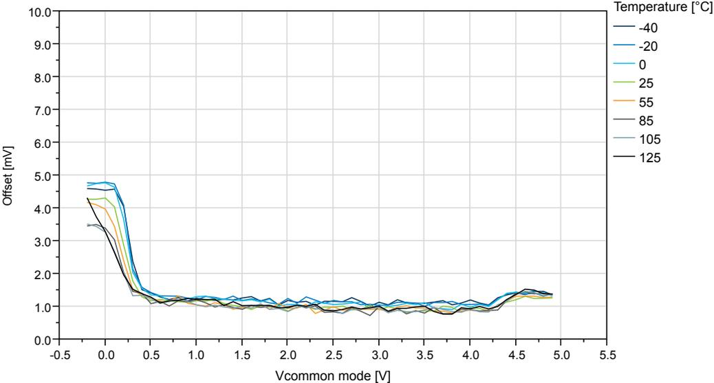
Figure 35-69. Offset vs.  $V_{CM}$  - 10mV to 50mV ( $V_{DD}=5V, T=25^{\circ}C$ )
