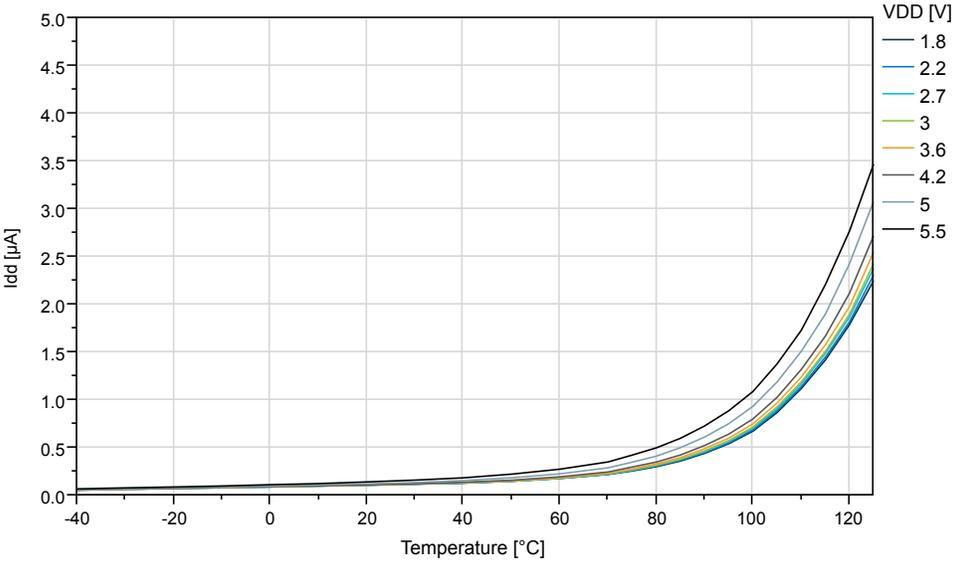
Figure 35-26. ATtiny814: Power Down Mode Supply Current vs. V<sub>DD</sub> (all functions disabled)
