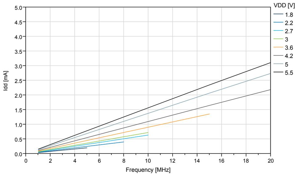
**Figure 35-7. ATtiny214/ATtiny414: Idle Supply Current vs. Low Frequency (0.1-1.0MHz) at T=25°C**
