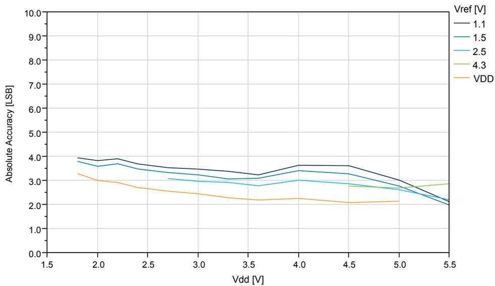
Figure 35-57. Absolute Accuracy vs.  $V_{ref}$  ( $V_{DD}=5.0V$ , 115kps)
