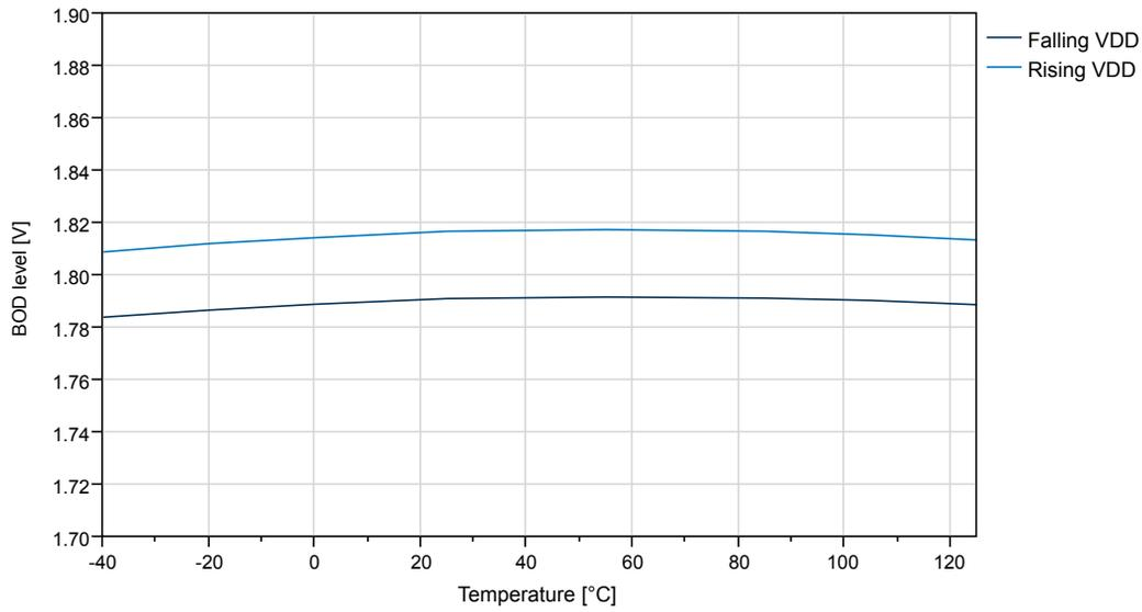
**Figure 35-54. BOD Threshold vs. Temperature (Level 2.6V)**
