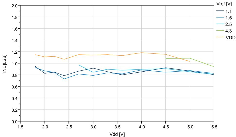
**Figure 35-63. INL vs.  $V_{ref}$  ( $V_{DD}=5.0V$ , 115kps)**
