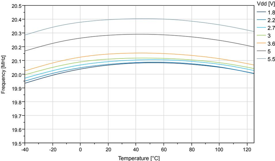
Figure 35-73. OSC20M Internal Oscillator: Frequency vs.  $V_{DD}$
