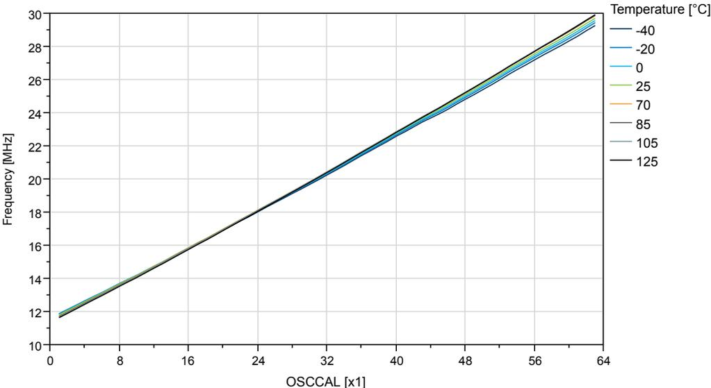
Figure 35-72. OSC20M Internal Oscillator: Frequency vs. Temperature
