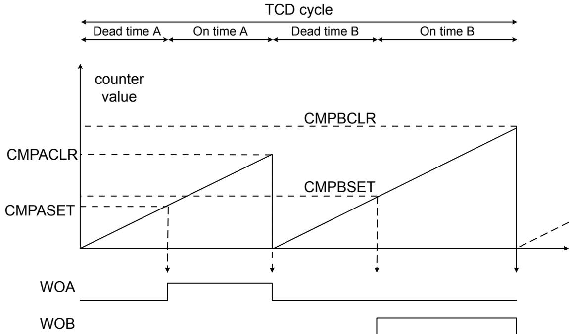
In the figure above,  $CMPASET < CMPACL R$  and  $CMPBSET < CMPBCLR$ . This causes the outputs to go high. There are no restrictions on the  $CMPASET/CLR$  compared to the  $CMPBSET/CLR$  values.
