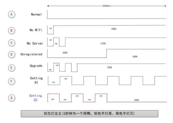
The flashing of the Wi-Fi status light is in a cycle of 2 seconds, as shown in the figure, the low-level light is on and the high-level light is off. Detailed explanation of each status:
