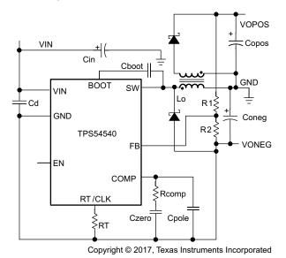
Figure 34. TPS54540 Split Rail Power Supply
