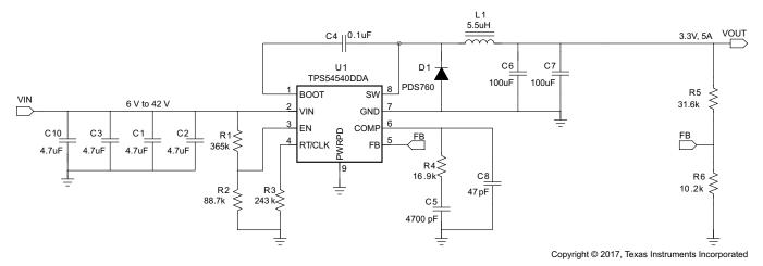
Figure 35. 3.3 V Output TPS54540 Design Example
