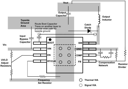
Figure 58. PCB Layout Example
