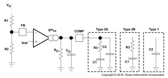
Figure 31. Types of Frequency Compensation
