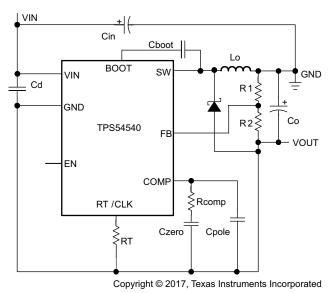
Figure 33. TPS54540 Inverting Power Supply
