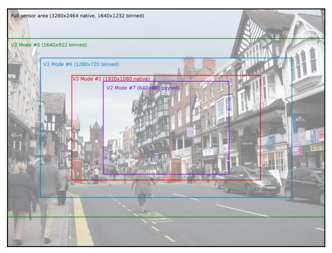
You can manually select the sensor's mode with the *sensor\_mode* parameter in the PiCamera constructor, using one of the values from the # column in the tables above. This parameter defaults to 0, indicating that the mode should be selected automatically based on the requested resolution and framerate. The rules governing which sensor mode is selected are as follows:
