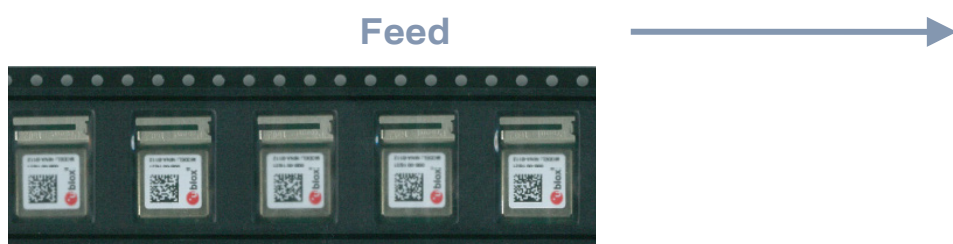
Figure 8: Orientation of NINA-W132 module on tape
